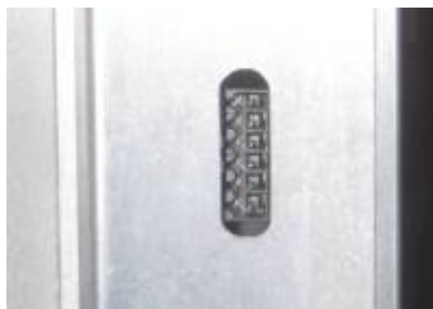
LEFT side connector shown for the 3 Manual Pushbuttons. Insert the connectors until they lock (click) in place.
